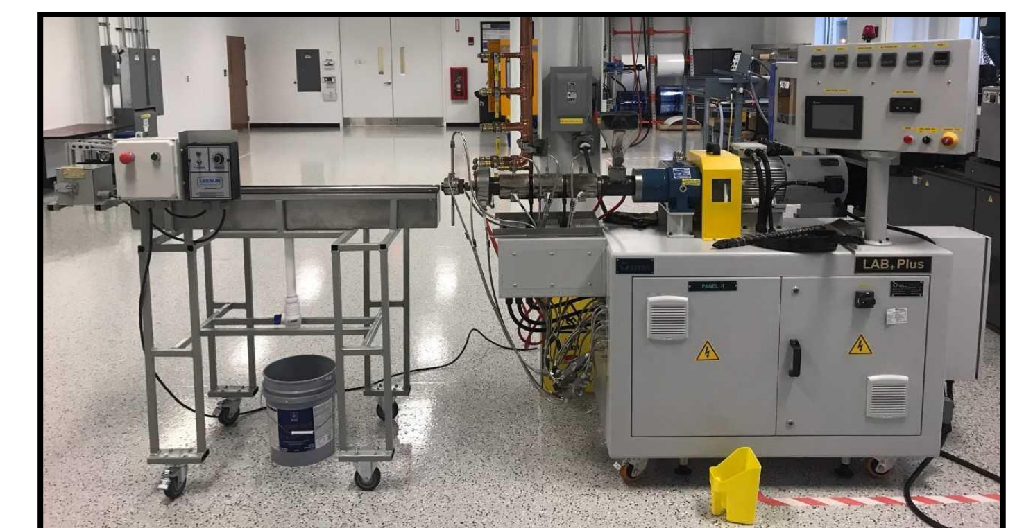
Figure 13: Cooling Line System Actual Set-up
