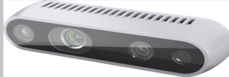
Figure 1: Image of the intel real sense camera used for vision tracking
