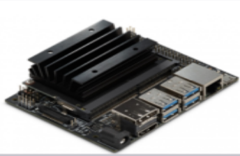
Figure 2: Image of the Nvidia Jetson Nano computer. This is used for all the GPIO and computation of scripts.
