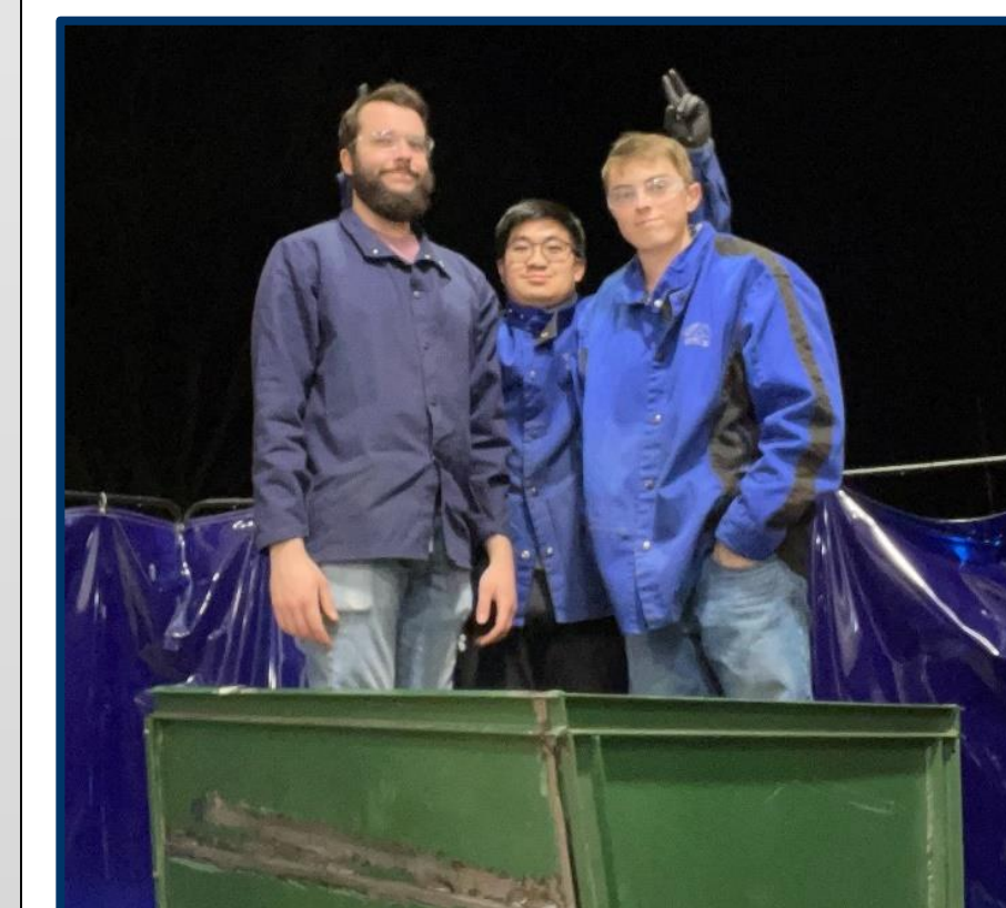
Figure 9: Load Testing: Students Standing in Hopper ~450 Lbs.
