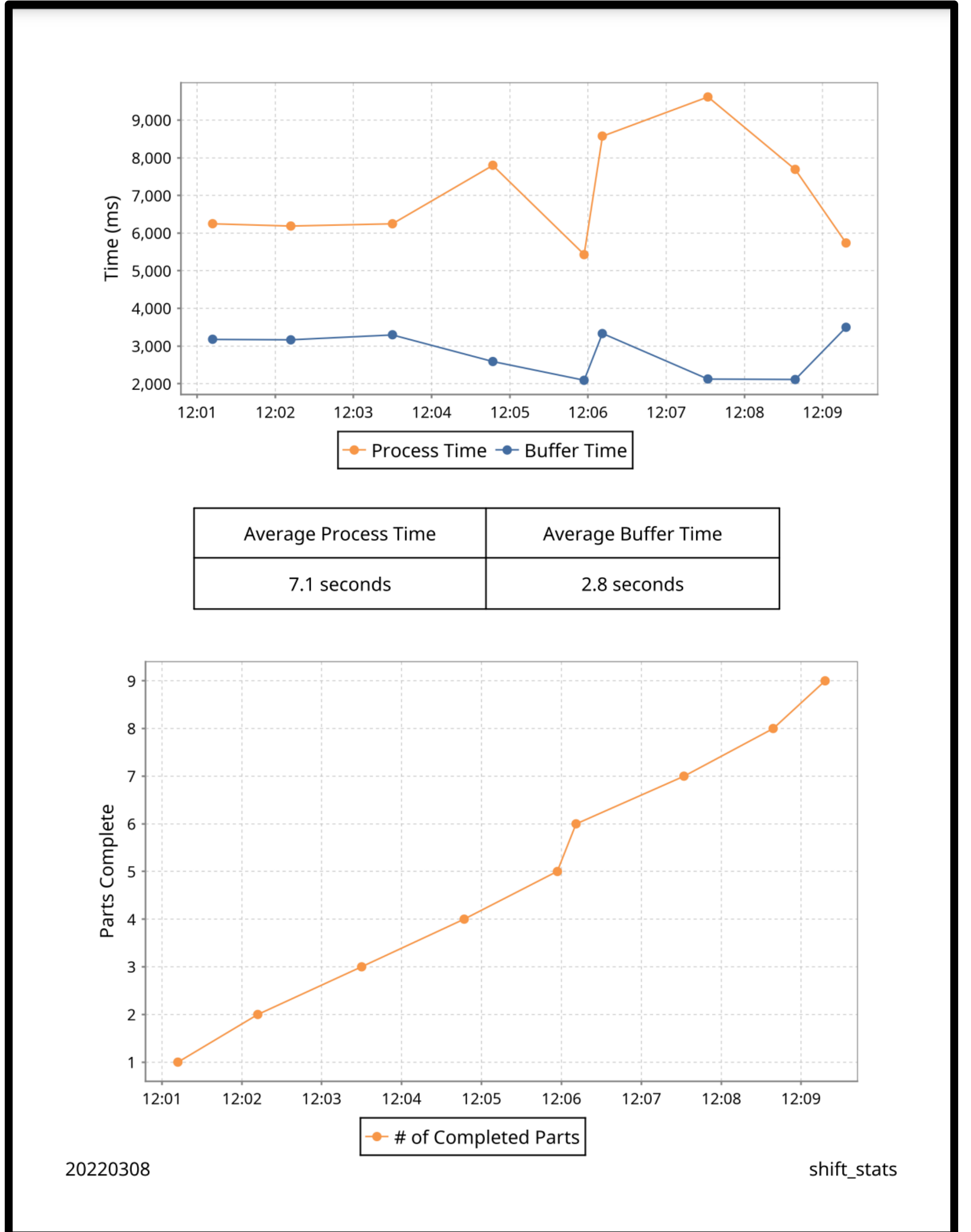
BELOW: Example report generated in Ignition showing takt time graph and output over the day.
