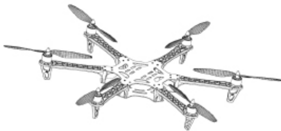
Figure 1: Hexacopter Current Design with Fixed Arms
