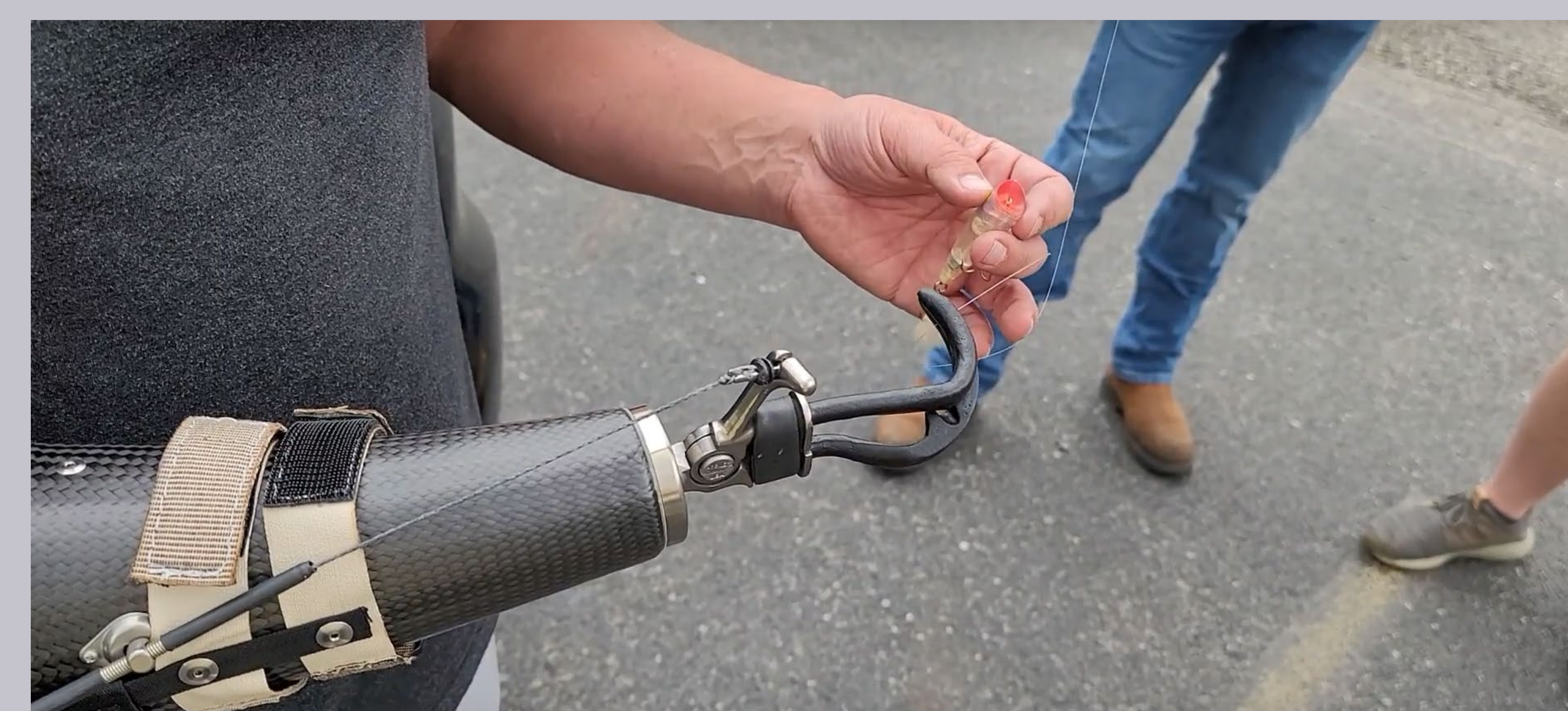
Figure 5: Challenger using modified fishing prosthetic with coated grips to tie knots and practice tying lures on fishing line.
