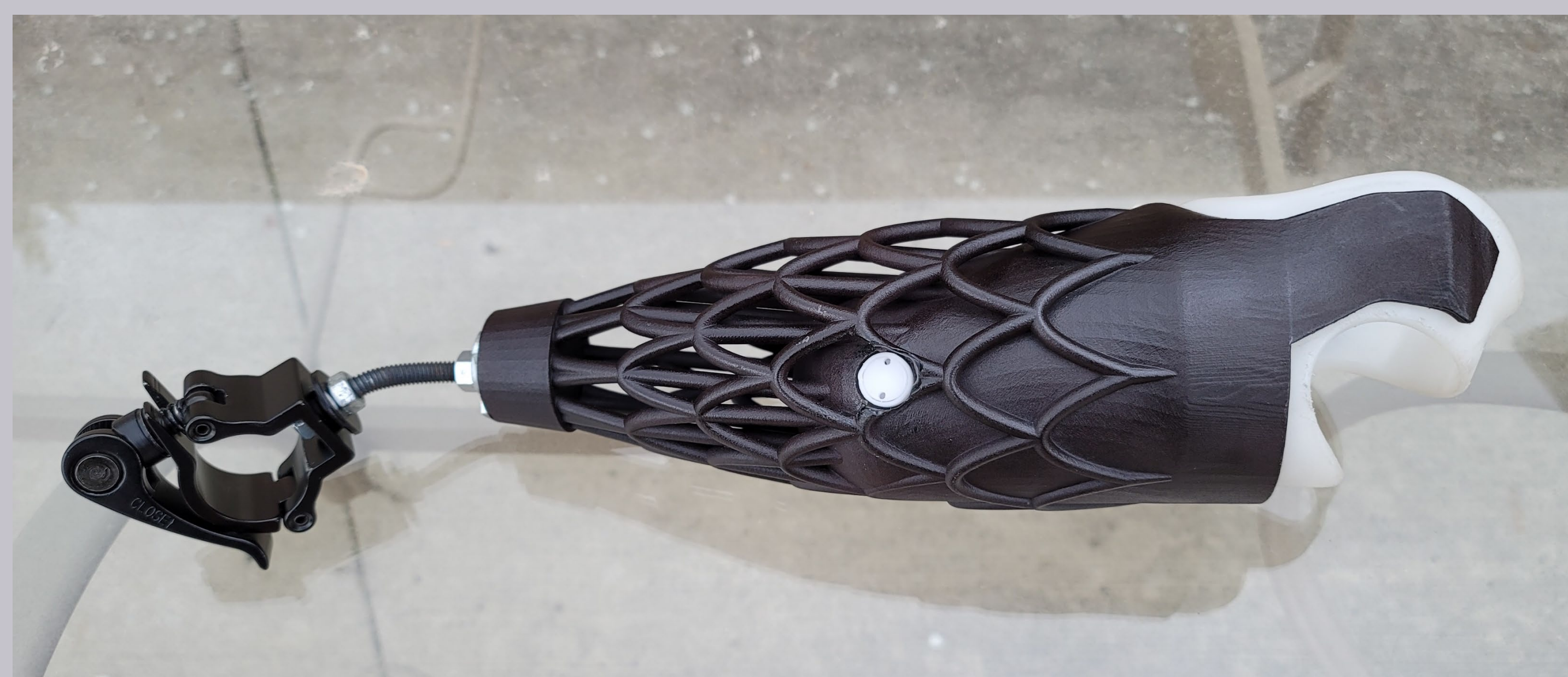
Figure 3: Close up of archery prosthetic with visible releases and quick release truss.
