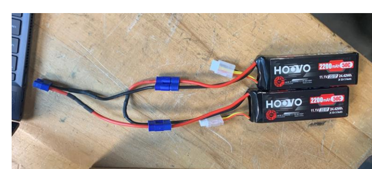
Figure 9: 11.1V(2) LI-PO wired in series
