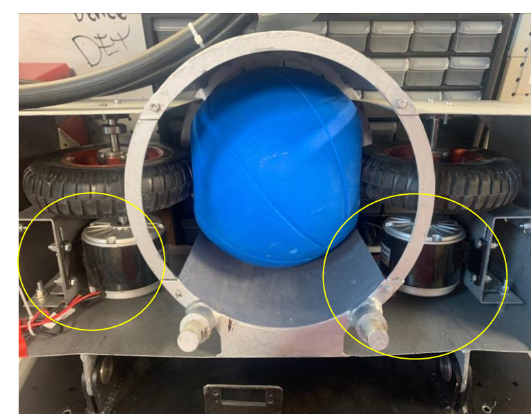
Figure 10: Two 24VDC Permanent Magnet Motors
