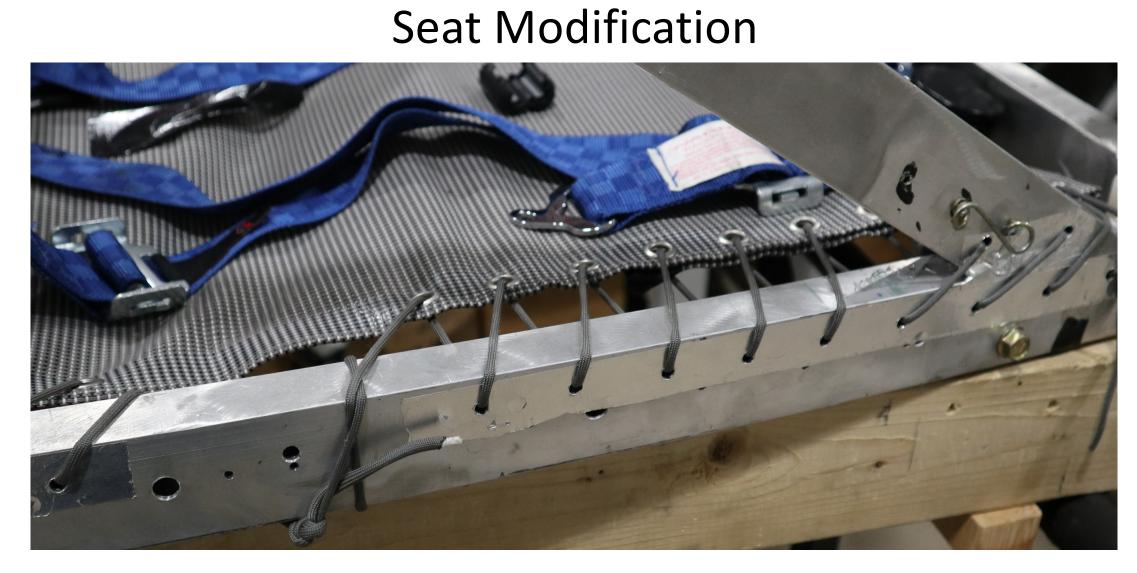
The seat also required multiple iterations of redesign and testing. The redesign including determining the location and method of attachment to the vehicle frame as well as the material the seat should be made of rather than the existing aluminum sheet. Prior to the impact of COVID-19 the team was working to find a solution for the seat, however there was no time to manufacture and complete the changes.
