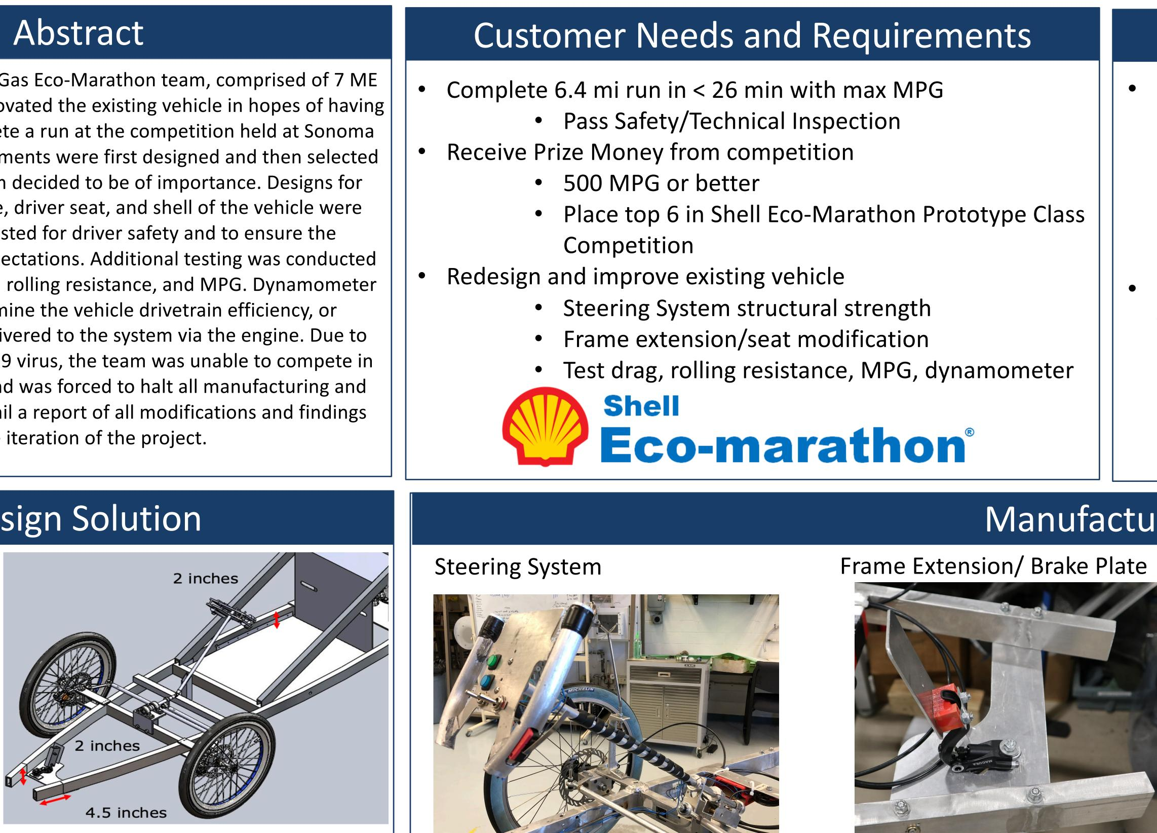
**Left:** Butterfly Steering Wheel Design with attached brake handle and throttle. The design also includes testing with a prototype the driver used to determine best button/switch layout. **Above:** Vehicle frame/seat modifications to allow for the driver and the team to pass technical inspection **Top Left:** Comparison of old bearing mount for steering system support versus redesigned steering system bushing mount. Reduced weight and provided better structural support.
