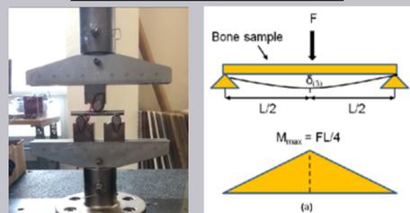
The purpose of this testing procedure was to conduct a 3-point bend test on aluminum A360, steel, and brass metal rods of the relatively same diameter to pick the optimal material choice for the shear pins that will be used for the final Zimmer Biomet fail-safe design.
