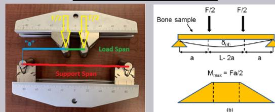
The goal of this testing was to develop a procedure for four-point bend compression testing of the shear pins for the improved fail-safe design. Due to the samples bending into contact with the fixtures before fracture and equipment failures, a switch to three-point bend testing was made for the next round of testing.
