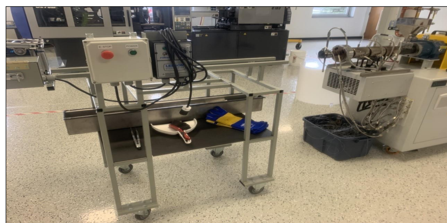
Figure 1: Extruder and Cooling Assembly
