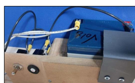
Figure 9: Battery Inside Housing
