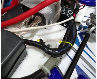
Kelly KDZ controller Mounted underneath the steering column
