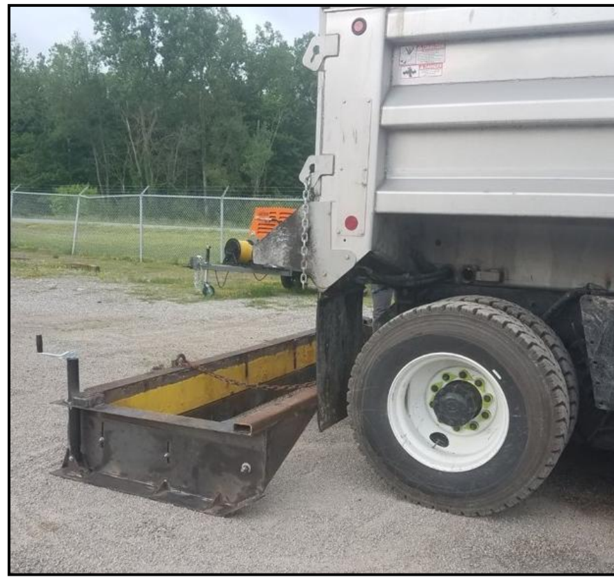
Figure 2: Paver Attached to Truck
