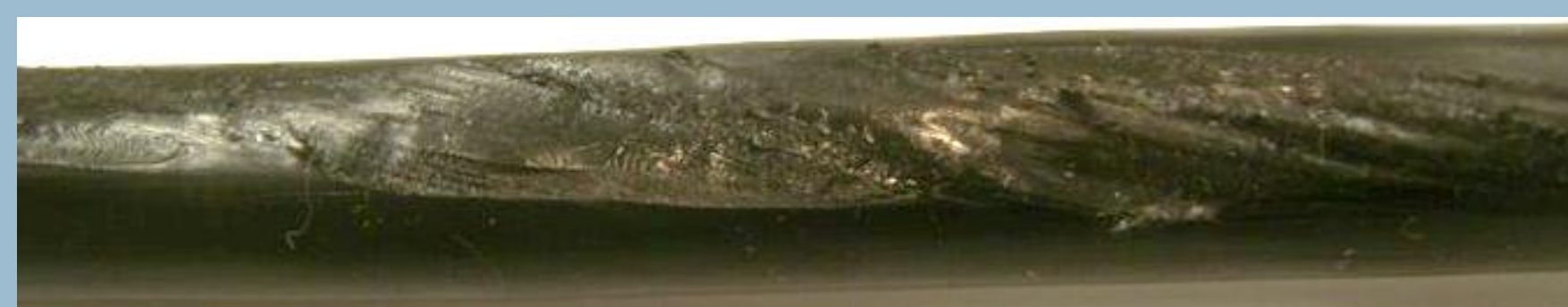
Scoring caused by cable installation.
