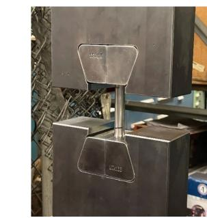
Tensile testing was performed at Metal Technologies in Auburn, IN. MTI received the as-cast tensile specimens, machined them to specification, and pulled them on their tensile testing machine (left).
