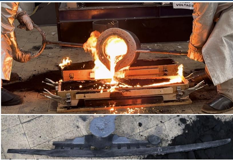
Green sand molds were packed and poured at the Trine University Foundry. Three iteration of the sword were cast in steel. The rough as-cast surface finish was ground smooth. Excess material and flash was also removed during this time. 3 swords were ground to the desired weight and shape.
