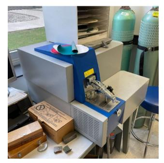
Hardness testing was performed using a LECO LR310 Rockwell Hardness Tester (right). This machine applies a large load on the specimen with the necessary indenter to determine the hardness of the material.
