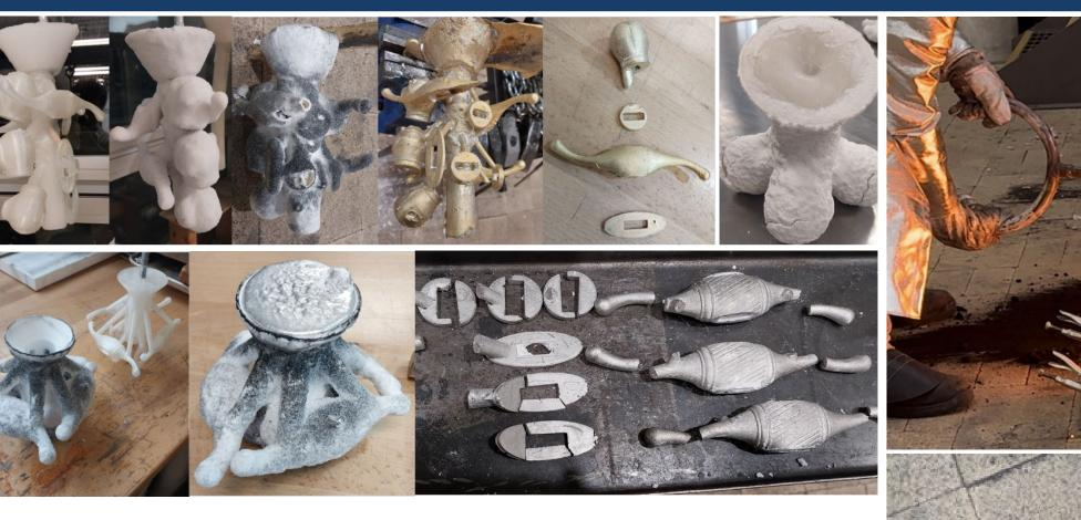
The sheath cap, guard, transition piece, and lion head pommel were cast using investment casting with Polymaker polycast filament, allowing for flexibility in design adjustments. These parts were cast using metals such as brass, tin-bismuth, and zinc, with careful attention to gating, burnout, and pour quality to reduce defects. After casting, each piece was cleaned, polished, and finished to achieve desired appearance for later assembly.
