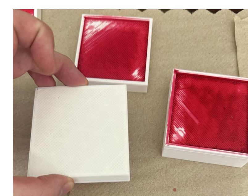
Figure 14. Dye penetration results on 3D printed (ABS) specimen
