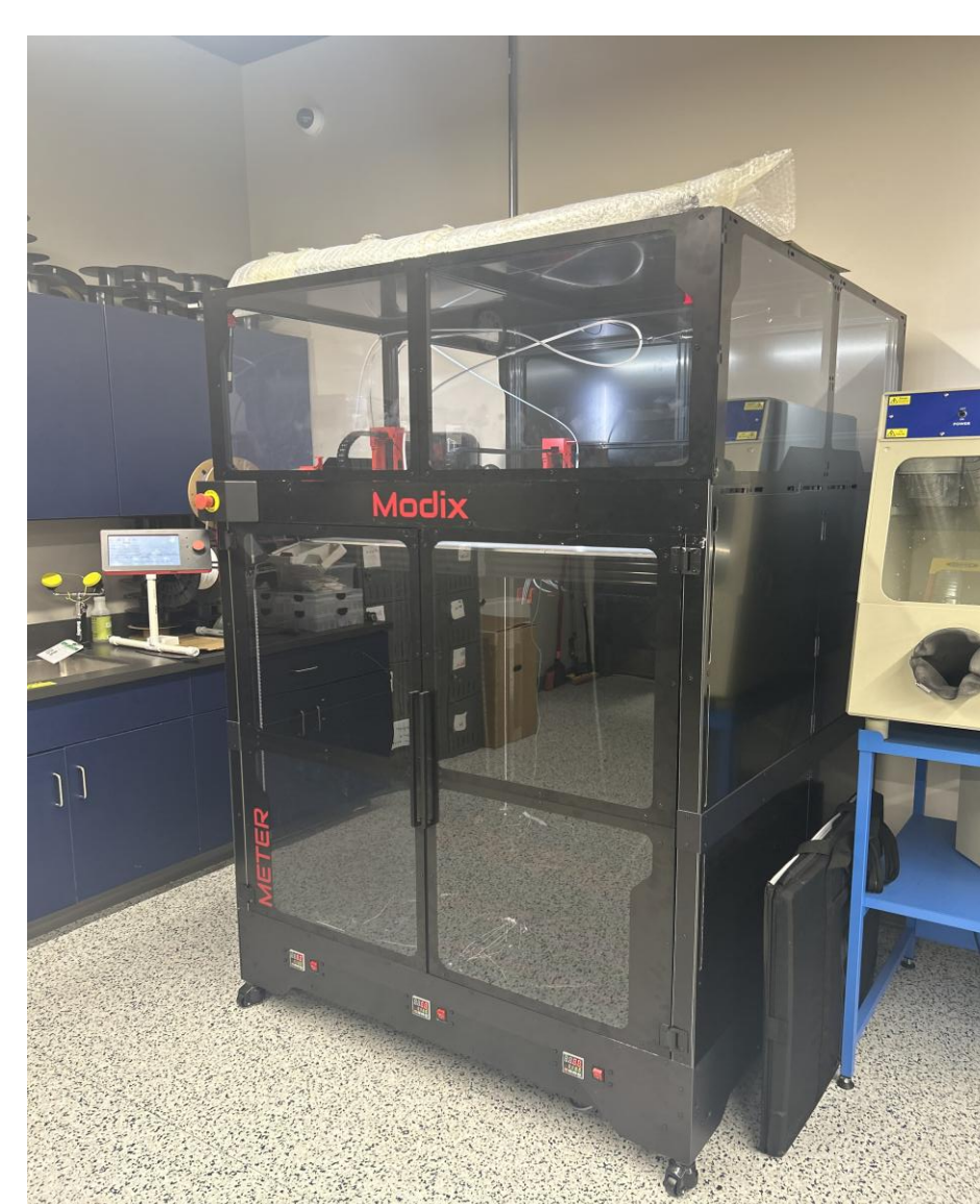
Figure 5. Modix Big-Meter manufactured the lid and bottom insulation chamber
