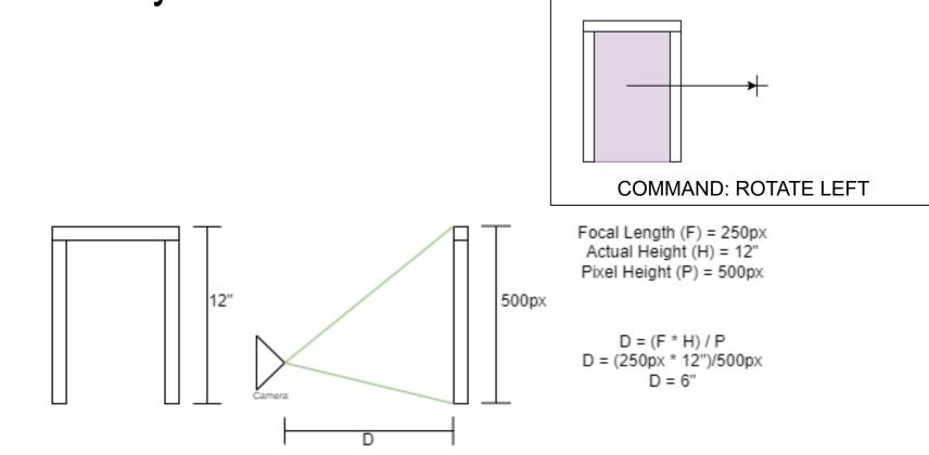
Additionally, this vision system is able to estimate the distance from the camera to the receiver. Because the size of the reflective tape shape is known, we can use the focal length of the camera, the pixel measurement of the shape, and the actual dimensions of the shape to calculate the distance. This is useful for determining the power with which to pass.
