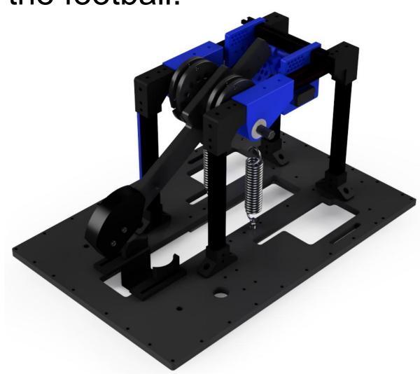
A latching mechanism is needed to safely and securely hold the kicking leg in place and release it when directed. Utilizing two servo motors, the team created a cam and follower mechanism, improving the mechanical advantage by 1.75 times. As the cam rotates counterclockwise, it unhooks from the latch component, pushing it away, releasing the leg. This mechanism does not require power to hold the arm.
