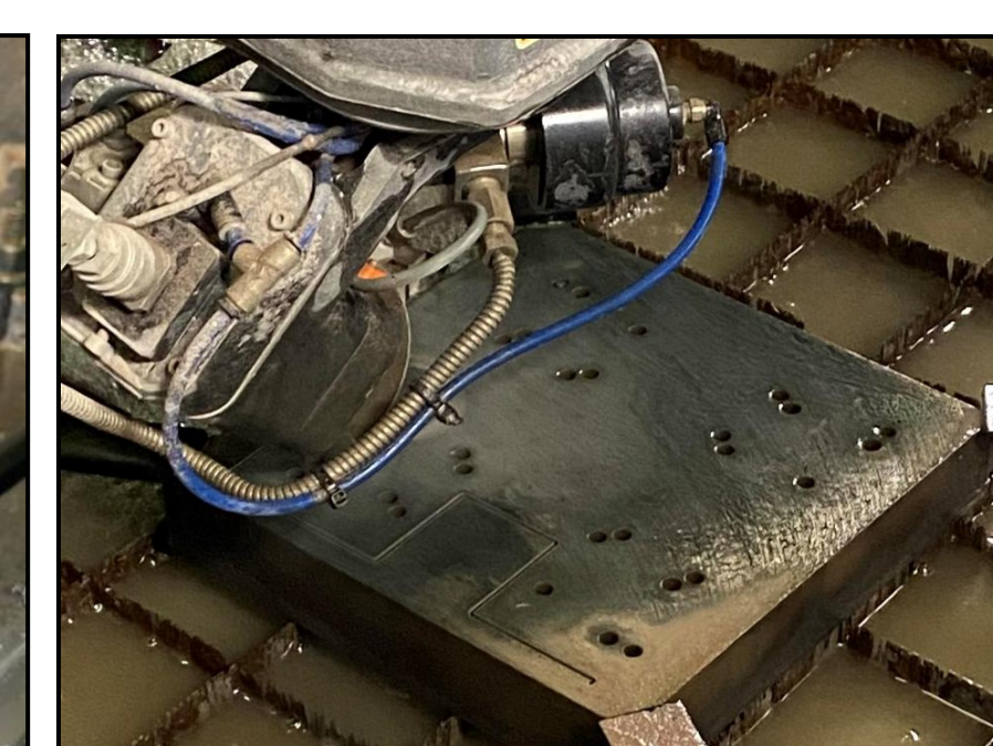
Figure 13: Slot-Mod Base Waterjet-Cutting
