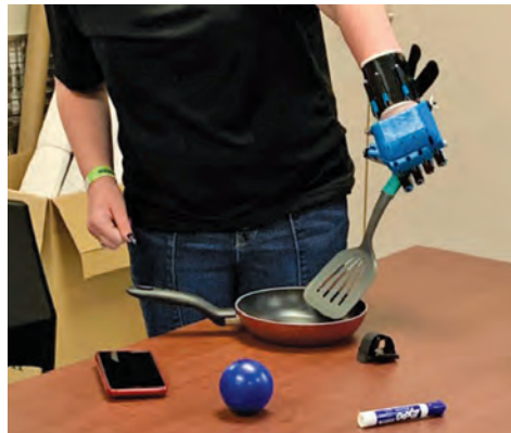
One of the recipients of prosthetic hands designed and 3D printed by a group of Trine University seniors performs validation testing with the device. The girls open and close fingers on the prosthetic by flexing their wrist.
